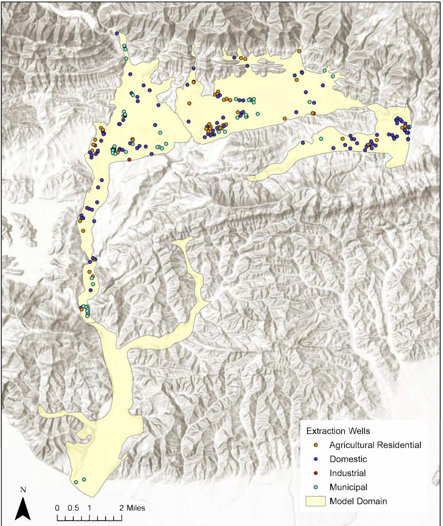
Figure 16. Modeled Extraction Wells and Well Categories
