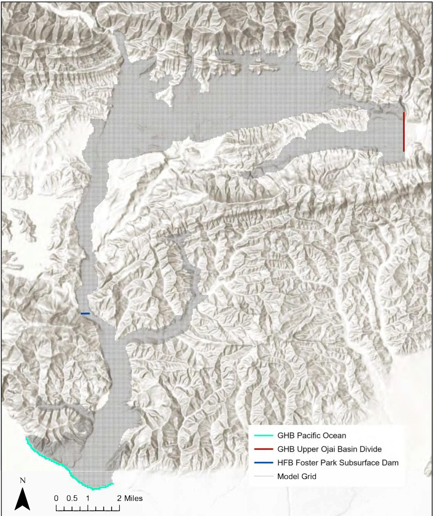
Figure 8. General Head Boundaries (GHB) and Horizontal Flow Barrier (HFB) Locations
